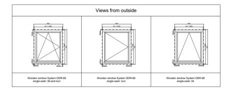
Parameters of wooden reference window (single-sash window 1230x1480mm) Glazino Resistance to wind load TET (g) System Uw Ug LT Rw ackage DDR-68 4x16x4 1.3 1 0.5 0.68 NPD 7A 4 33dB 0,6 0,53 0.74 DDR-78 4x14x4x14x4 0,95 NPD E900 4 34dB DDR-92 4x16x4x16x4 0.83 0,5 0,38 0,59 NPD 5A 34dB 4 Ug - heat transfe fficient of the glazing package. TET(g) - solar energy tr LT - light tr
